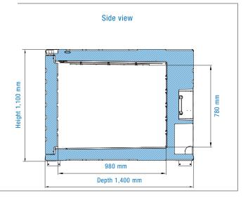
Refrigerated container with metal feet: transportable by pallet jack or forklift
